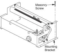
Figure 11 - Attaching Base Assembly to Fireplace Floor
